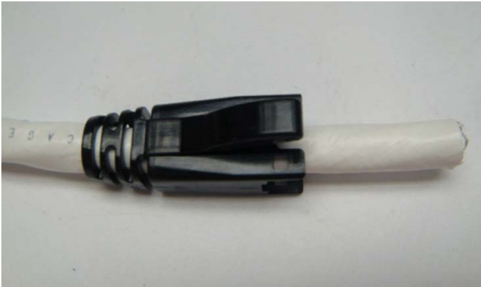
Figure 6: Attaching the strain relief grommet
